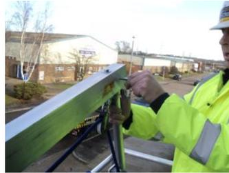
To fit the Support Tubes remove the Locking Pin from each end of the Lifting Beam, insert the Support Tube into the large hole on the underside of the Lifting Beam and replace the Locking Pin to secure.
