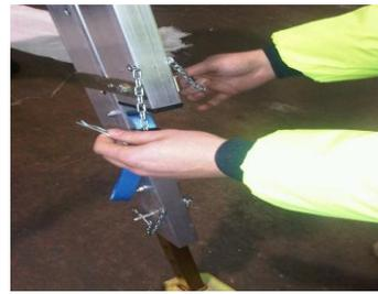
Adjust the height by removing the two Leg Pins and pulling on both Leg straps rolling the Window-Dec Platform up the wall to the desired height and replace both Leg Pins remembering to also replace the safety 'R' Clips provided. After adjusting to height it will be necessary to re-level the Window-Dec Platform by moving the feet either away or towards the wall.
