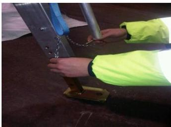
The Feet maybe adjusted in 25mm increments but in extreme cases either Leg can be adjusted Independently. Fit Pin and 'R' Clip to secure.
