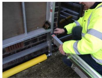
Fit both Legs using the Pins and 'R' Clips provided and ensure that the Pins are inserted outside in, to minimise the risk of the 'R' Clips being Knocked out. **REMEMBER:** Fit the Legs to the 'Normal use' hole Labelled on the underside of the platform.
