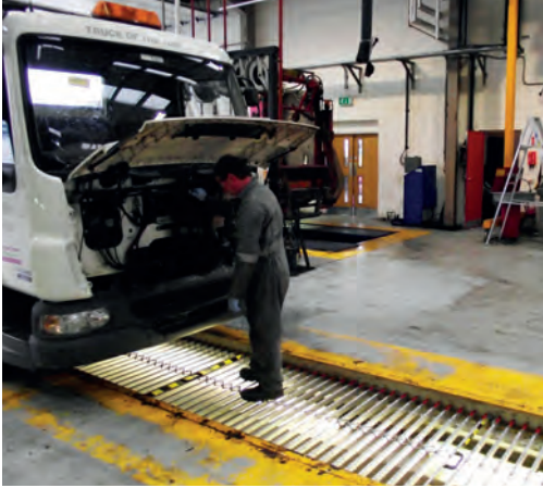
Robust yet lightweight inspection pit covers are easy and quick to deploy to protect pits.
